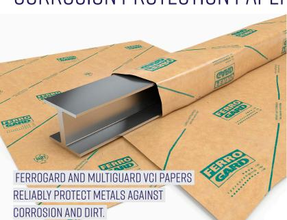
Ferrogard and Multiguard VCI corrosion protection papers are high quality kraft papers which constantly release small amounts of corrosion protection active ingredients (VCI: Volatile Corrosion Inhibitor), thus effectively protecting metal components from corrosion during transport and storage.
